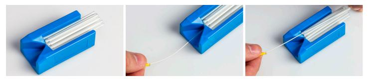
Loading a protection sleeve onto a fiber can be tedious, even for the most experienced technicians. Plus, if they have physical impairments such as poor eyesight then it can become nearly impossible. Designed to make loading protection sleeves onto fiber quick and easy, the QuickSleever protection sleeve insertion tool is ideal for aligning fiber to the holes of protection sleeves and is a real timesaver. This protection sleeve insertion tool features the following:
