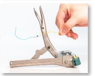
This vise-style MR1 hand tool is designed to crimp various AMP Picabond connectors onto 19 - 28 AWG wires. This crimper also features the following:
