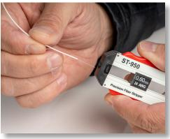
Designed for precision fiber optic stripping, this tool is perfect for stripping the 600 - 1100 micron buffer coating to expose the 250 micron acrylate-coated glass fiber of fiber optic cables. This precision fiber stripper also features the following:
