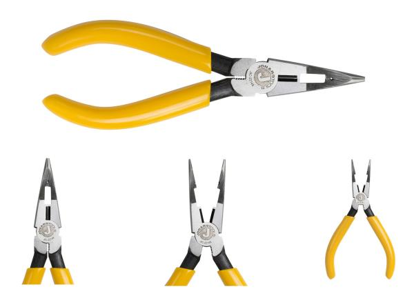
Jonard's long nose pliers are made of heat treated chrome vanadium steel with induction-hardened cutting edges for maximum strength and durability. These long nose pliers feature the following:
