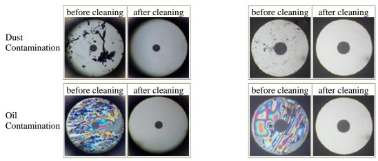
mechanism of cleaning MPO/MT-RJ connectors with pins.
